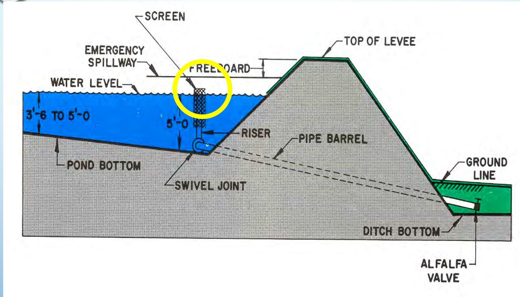
Diagram of catfish pond standpipe and drain
