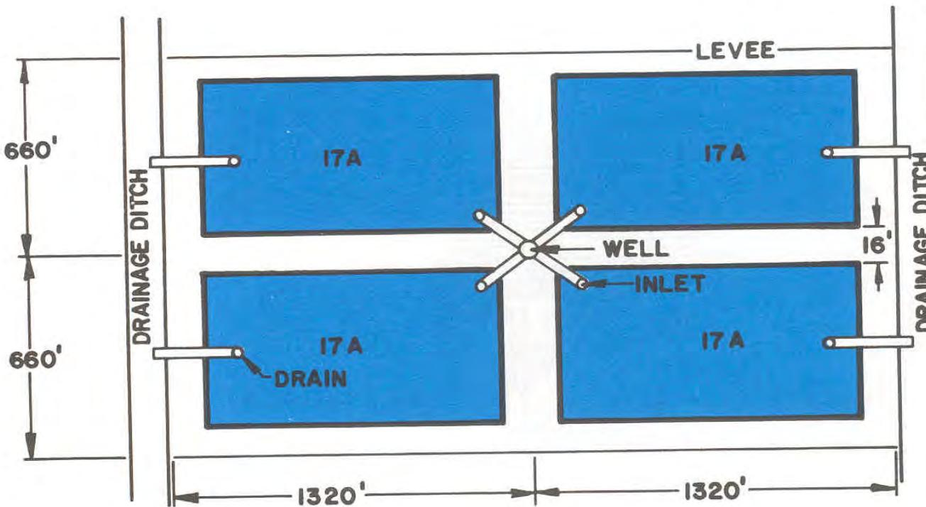
Diagram of a catfish levee pond (upper) and pond layout (lower)
